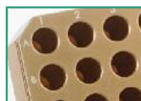
Alphanumeric identification of wells facilitating tube location
