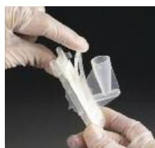
Clip top of funnel and base together.
