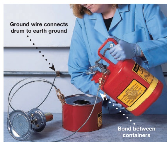
Bond dispensing can to receiving container, then ground receiving container to a water pipe or ground strip.
