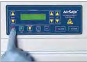
AirSafe™ Cyano automatic safety controller monitors all functions of the cabinet including humidity levels, filter conditions and airflow
