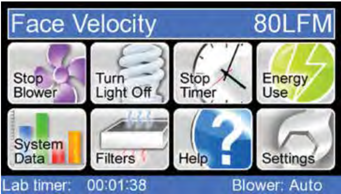
AirSafe NXT home screens allow monitoring and control of all ductless hood features
