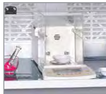
High mass polypropylene construction for balance stability
