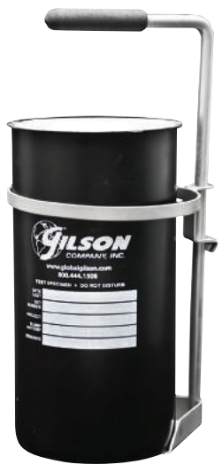
HM-161 shown with 6in concrete cylinder
